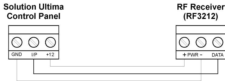
Figure 1: RF Receiver (RF3212) Wiring Diagram
